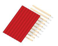
better in the summer. Adding metal directly over shingles would corrode the metal and cause the paint to degrade.
